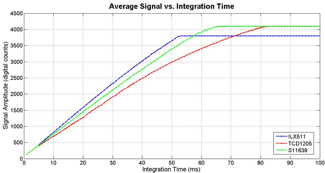
Figure 1: Signal level as a function of integration time for each sensor: the ILX511B (blue), the TCD1205DG (red) and the S11639 (green). The plots for the S11639 and S11639-01 are visually the same.
