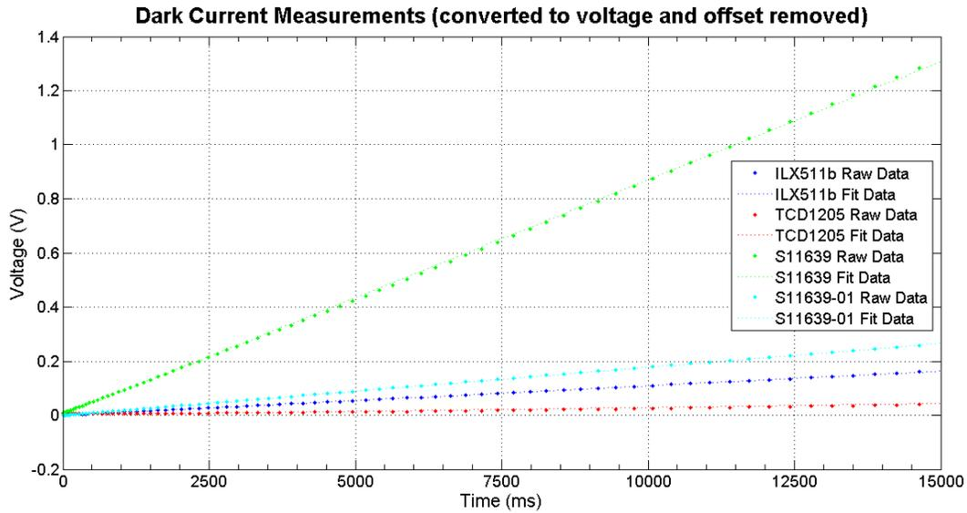
**Figure 2:** Dark output level in volts for each sensor (ILX511B, TCD1205DG, S11639 and S11639-01) as a function of integration time, including the linear fit curve. In this plot the digital counts have been converted to a voltage, and the initial offset has been removed.
