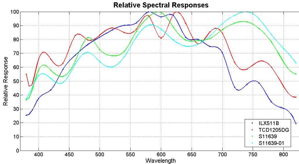
Figure 3: Relative spectral response of the Sony ILX511B, Toshiba TCD1205DG, Hamamatsu S11639 and S11639-01.
